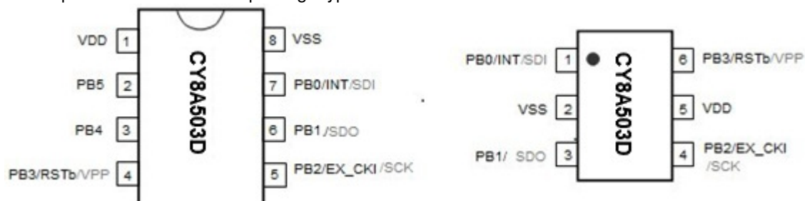
Figure 1 Package pin assignment
